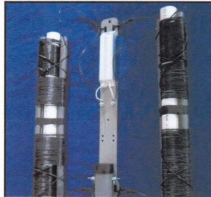
Folded terminated dipole components; various models will vary in size.
